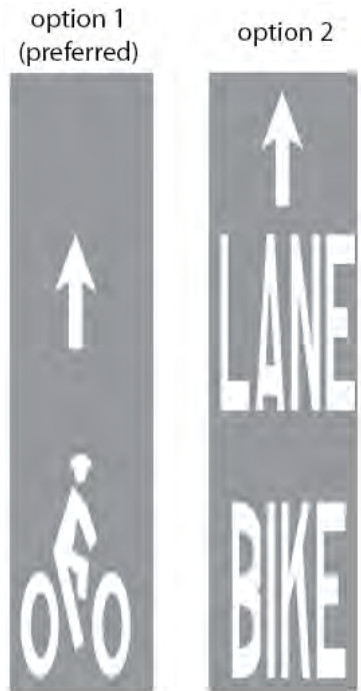
Bike Lane Pavement Markings
