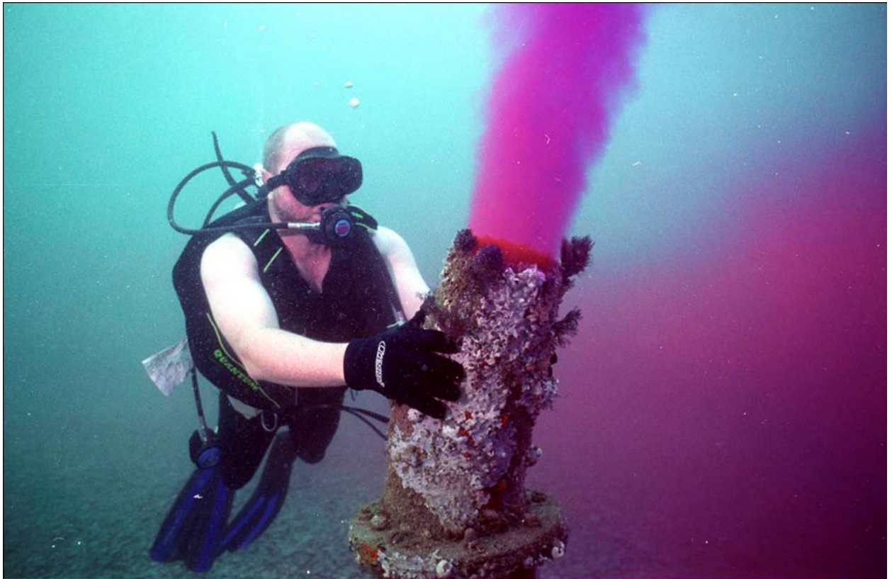
Figure XX An outfall diffuser nozzle at a desalination plant in Perth, Australia expelling concentrate colored with a red dye for a salinity dispersion test.
