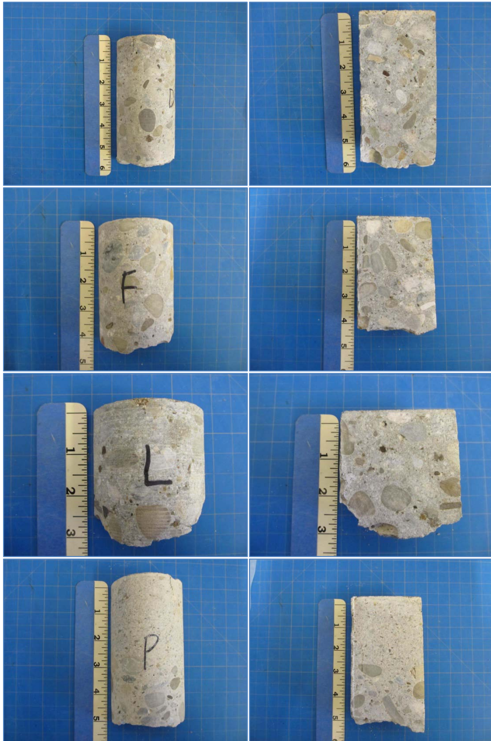
Photo 1. Core samples as received. The photo on the right is the sawn-cut face of the core sample shown to the left.
