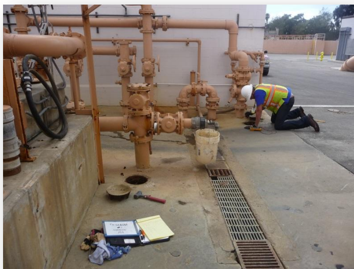
Photo 8) Cathodic Protection Testing at Waste-Water Treatment Plant
