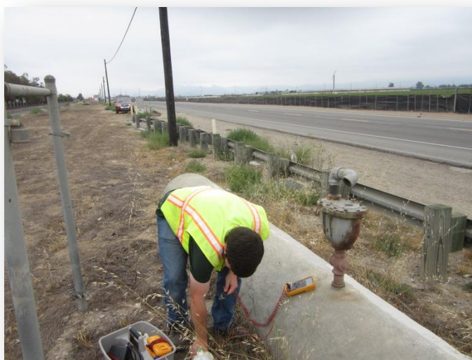
Photo 1) Measuring and Recording Pipe-to-Soil Potentials on a Pipeline
