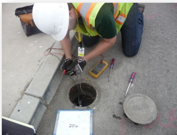
Photo 7) Cathodic Protection Testing at Waste-Water Treatment Plant
