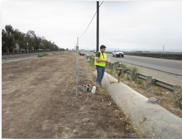
Photo 4) Cathodic Protection Testing on Oxnard Conduit
